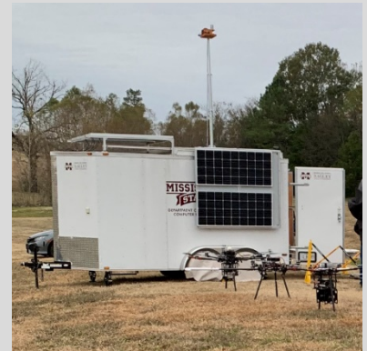
Pictures: [Top] Artistic view of NASA's CYGNSS satellite, and [Bottom] droNE_Station (NEST) that serves to house, energize, and deploy the UAS-based sensing system conveniently across multiple testing areas. Subset of lab's UASs with sensor modalities
